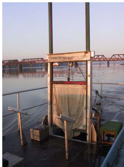
Figure 9: Schematic diagram of the vertical-sampling trap (top) (reprinted from Vernon 1966). The surface net (bottom left, located on the upstream end of the trap), is fished simultaneously with the depth-sampling net (bottom right, shown in the raised position), in order to measure the proportion of surface migrants to migrants at depth. The Mission railroad bridge can be seen in the background (downstream) of the photo at right.
