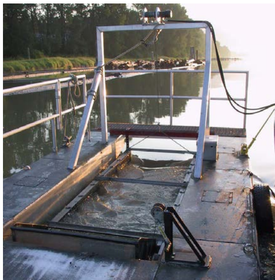
Figure 8: Mission Fraser River Pink Salmon fry sampling program. Schematic diagram of the inclined plane trap (top) (reprinted from Vernon 1966) and photos of the trap in the fishing (bottom left) and raised (bottom right) positions. Fry are entrained through the front of the trap, over a sloped screen, and into a holding pen at the downstream end.
