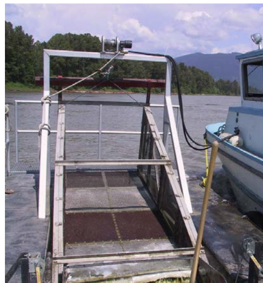
Figure 8: Mission Fraser River Pink Salmon fry sampling program. Schematic diagram of the inclined plane trap (top) (reprinted from Vernon 1966) and photos of the trap in the fishing (bottom left) and raised (bottom right) positions. Fry are entrained through the front of the trap, over a sloped screen, and into a holding pen at the downstream end.
