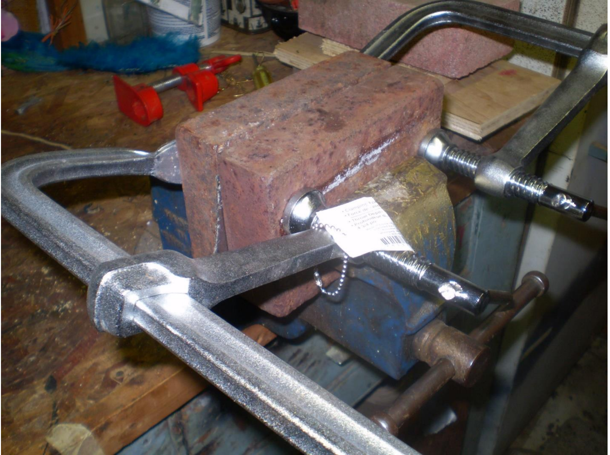
Photo 13: Pressing smolt scales using a bench vise.
