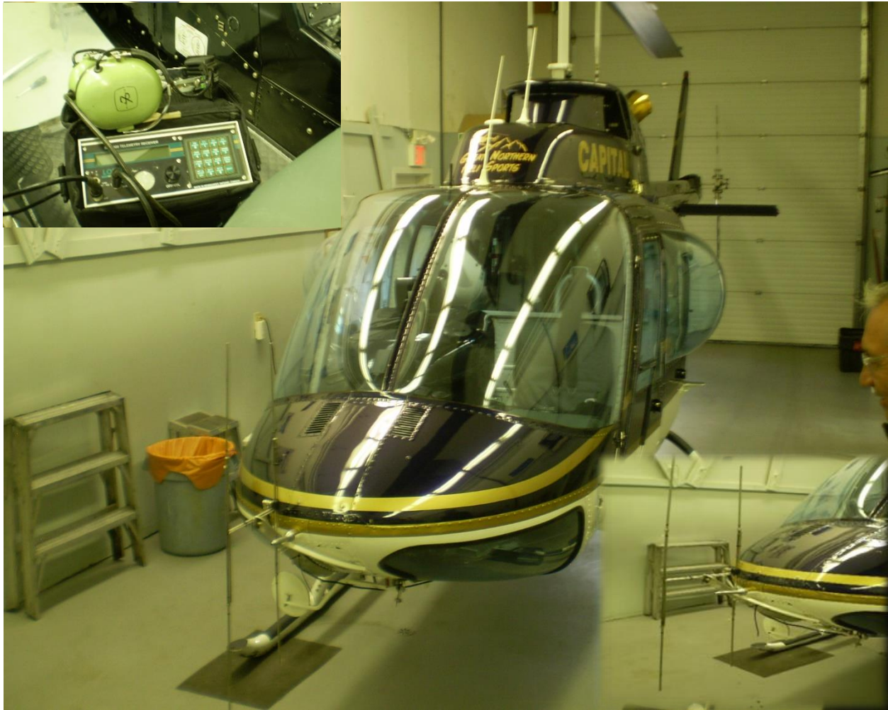
Photo 4: Helicopter Setup for Aerial Tag Detection.
