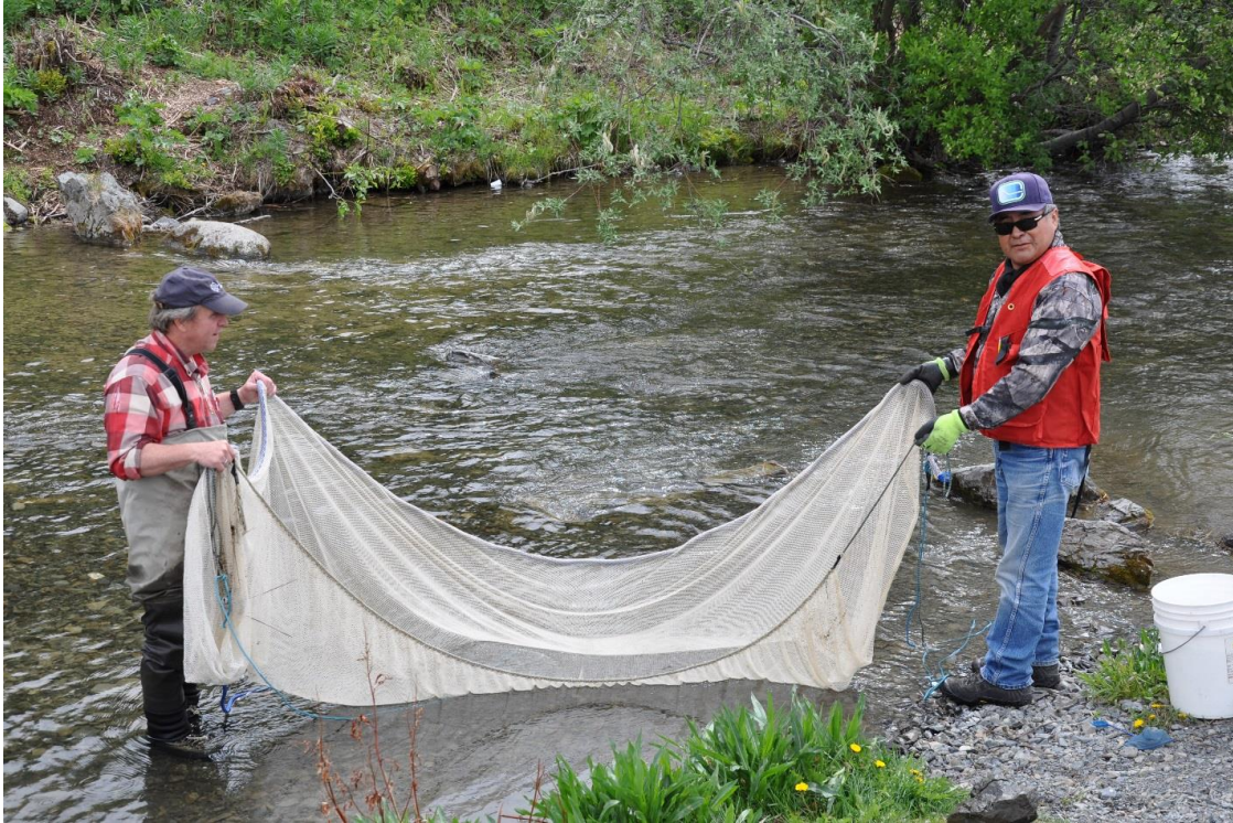
Photo 7: Beach seine used to capture juvenile salmon on Klukshu River and on Klukshu Lake. Picture taken May 18, 2016, at site C (Section 3.1), on the Klukshu River mainstem downstream of Vand Creek.
